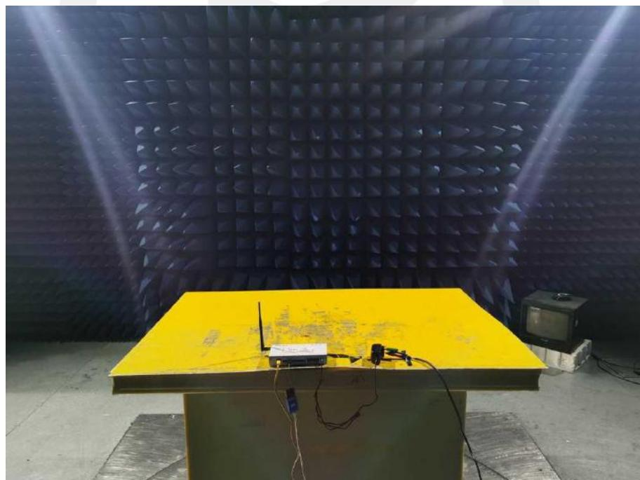
18.4.Photo of Radiation Emission Measurement ( Above 1GHz)
